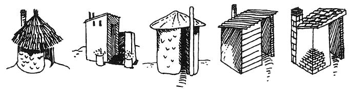
Ventilation is provided in VIP's by a vent pipe with yproof netting at the top.
