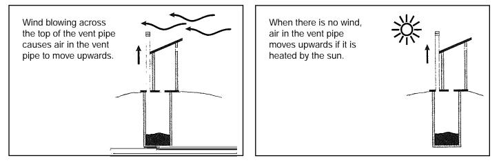
The upward movement of air in the vent pipe reduces nuisance from smells and insects.
